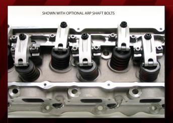
STEP 4: LUBRICATE THE TIPS OF THE INTAKE AND EXHAUST PUSHRODS USING THE SUPPLIED HIGH PRESSURE LUBE. INSTALL EACH ROCKER ARM WHEN THE CAM LOBE IS ON ITS BASE CIRCLE AND TORQUE THE 5/16-18 X 1.250" SHAFT BOLT TO PROPER SPEC. NEVER TORQUE SHAFT BOLTS WHEN THE ROCKER IS UNDER ANY SPRING LOAD AS SHAFT DAMAGE MAY OCCUR. RETORQUE ALL MOUNTING HARDWARE AFTER INITIAL BREAK-IN.
