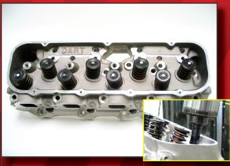
STEP 1:-THE-CYLINDER HEAD MUST BE MACHINED PRIOR TO INSTALLING THIS KIT. IF YOUR HEAD HAS NOT BEEN MACHINED, PLEASE FOLLOW DIRECTIONS FOUND ON INS-24017. JESEL CAN PERFORM THIS MACHINING OPERATION FOR YOU IF NEEDED.
