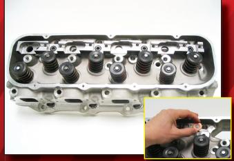
STEP 2: LOOSELY BOLT THE ONE-PIECE INTAKE STAND AND CHECK GEOMETRY USING THE AVAILABLE STAND HEIGHT CHECKING TOOL. IF THE STAND IS LOW, A SHIM KIT (KRS-28150) IS AVAILABLE TO RAISE THE STAND. IF THE STAND IS SITTING TO HIGH, THE HEAD WILL HAVE TO BE MILLED OR LASH CAPS MAY BE USED. ONCE THE CORRECT HEIGHT IS ACHIEVED, APPLY THREAD SEALANT TO THE INTAKE STAND BOLTS AND TORQUE TO SPECS LISTED ON PAGE 2
