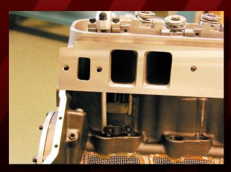
**STEP 3:** CHECK FOR PUSHROD TO CYLINDER HEAD INTERFERENCE AND CORRECT IF NEEDED. THE PUSHROD SHOULD NOT BE ALLOWED TO TOUCH THE HEAD OR BLOCK THROUGH ANY PORTION OF ITS TRAVEL. MEASURE FOR PUSHROD LENGTH NEEDED AND ORDER PUSHRODS. INSTRUCTIONS FOR MEASURING PUSHROD LENGTH ARE INCLUDED WITH PUSHROD LENGTH MEASURING TOOL **TOL-29450**.
