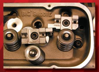
STEP 1: INSTALL INTAKE AND EXHAUST STANDS LEAVING 1/4-20 ATTACHING BOLT SNUG BUT LOOSE. APPLY THREAD SEALANT TO INTAKE BOLT AND OIL TO EXHAUST BOLT. TORQUE BOLTS TO 60-65 FT/LBS ON ALUMINUM HEADS AND 65-70 FT/LBS ON CAST IRON HEADS. USE THE LONGEST BOLT POSSIBLE FOR MAXIMUM THREAD ENGAGEMENT.
