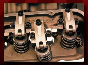
STEP 4: LUBRICATE THE TIPS OF THE INTAKE AND EXHAUST PUSHRODS USING THE SUPPLIED HIGH PRESSURE LUBE. INSTALL EACH ROCKER ARM WHEN THE CAM LOBE IS ON ITS BASE CIRCLE AND TORQUE THE 5/16-18 X 1" SHAFT BOLT TO 26-28 FT/LBS. NEVER TORQUE SHAFT BOLTS WHEN THE ROCKER IS UNDER ANY SPRING LOAD AS SHAFT DAMAGE MAY OCCUR.
