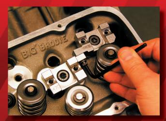
STEP 2: ONCE THE INTAKE AND EXHAUST STANDS ARE PROPERLY FASTENED, TORQUE THE 1/4-20 x 3/4" JOINING BOLT TO **12 FT/LBS**. IF THE STANDS ARE SHIMMED TO COMPENSATE FOR A LONGER LENGTH VALVE, THE STANDS MAY NEED TO BE MODIFIED TO SECURE THEM TOGETHER.
