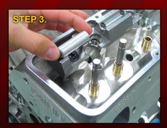
LOCATE AND PLACE THE ALUMINUM .561" DIAMETER CHECKER SHAFT ONTO THE ROCKER STAND.
