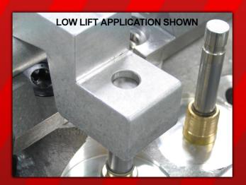
THE STAND HEIGHT CHECKER WAS DESIGNED TO OBTAIN PROPER GEOMETRY FOR A .600"-.800" VALVE LIFT APPLICATION.
