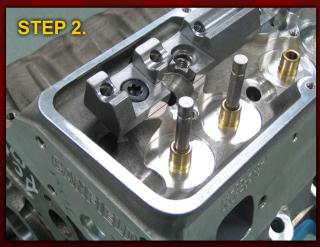
WITH THE PROPER INTAKE AND EXHAUST VALVE INSTALLED, BOLT THE ROCKER STAND TO THE CYLINDER HEAD WITHOUT USING ANY SHIMS.
