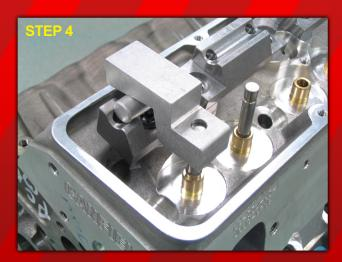
WITH THE VALVE IN THE CLOSED POSITION, SLIDE THE CHECKER OVER THE VALVE STEM AND ALLOW IT TO REST ON THE CHECKER SHAFT.
