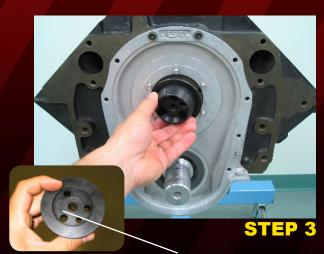
APPLY A THIN LAYER OF RTV SEALER TO THE RECESSED AREA ON THE CAM ADAPTOR.
