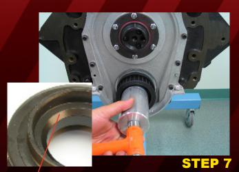
LUBRICATE THE CRANK SNOUT WITH A HIGH QUALITY ANTI-SEIZE COMPOUND.
