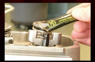
STEP 5: WITH THE LIFTER ON ITS BASE CIRCLE, PLACE THE CORRECT LENGTH PUSHROD INTO POSITION. APPLY SUPPLIED ASSEMBLY LUBE TO <u>PUSHROD TIP AND BOLT</u> ROCKER TO STAND.
