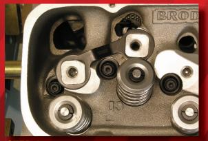
STEP 1: STARTING AT #1 CYL, PLACE STAND LINK ON INTAKE AND EXHAUST STUD BOSS. USE SUPPLIED SUPPORT WASHERS IF NEEDED TO SUPPORT STAND LINK. STAND LINK MAY BE ADJUSTED SLIGHTLY IF NEEDED FOR IMPROVED STAND ENGAGEMENT.
