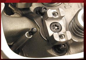
STEP 4: USING AVAILABLE ADJUSTABLE PUSHROD (TOL-29400), CHECK FOR PUSHROD TO HEAD INTERFERENCE AND CORRECT IF NEEDED. MEASURE FOR PROPER LENGTH PUSHRODS FOLLOWING INSTRUCTIONS INCLUDED WITH ADJUSTABLE PUSHROD TOOL.
