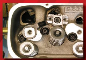
STEP 2: LOCATE INTAKE STAND NEEDED FROM CHART ON BACK PAGE. USE LONGEST BOLT POSSIBLE AND INSTALL USING THREAD SEALANT. DO NOT TORQUE STAND BOLT AT THIS TIME.
