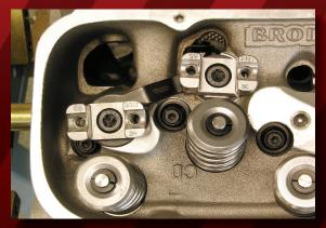
STEP 3: LOCATE EXHAUST STAND NEEDED FROM CHART ON BACK PAGE. USE LONGEST BOLT POSSIBLE AND INSTALL USING ENGINE OIL ON THREADS. CHECK TO MAKE SURE BOTH STANDS ARE ENGAGED INTO STAND LINK AND TORQUE BOLTS TO SPECS ON BACK PAGE.
