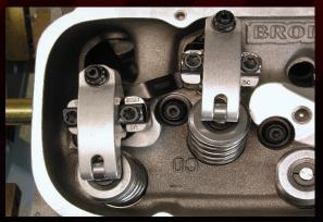
**STEP 6:** TORQUE ROCKER SHAFT BOLTS TO SPECS ON BACK PAGE. ROTATE ENGINE 90° AND REPEAT STEPS 5 & 6 FOR REMAINING CYLINDERS FOLLOWING ENGINES FIRING ORDER.
